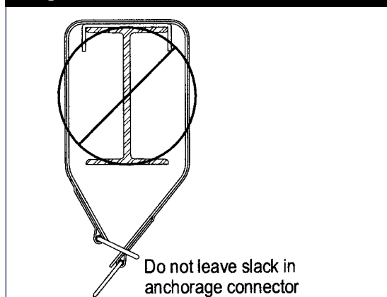
Figure 12 - Connecting to the Anchorage Connector
